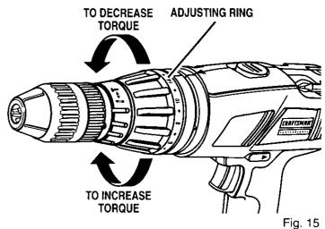
**Note:** Remember the two-speed feature (**HI-LO**) when setting torque. The amount of torque will vary depending on which speed setting you have your drill. Switching to **LO** speed will increase torque. Switching to **HI** speed will decrease torque.
